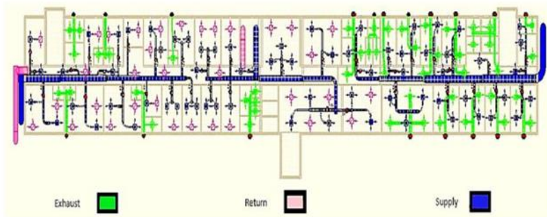
Figure (12) First Floor Duct Design
